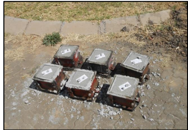
Concrete cubes for testing strength
